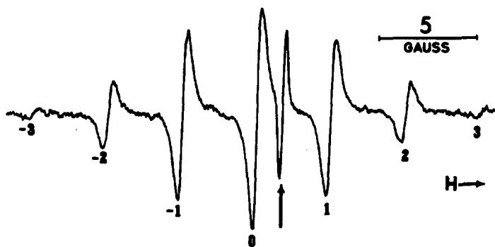
The hyperfine components of benzene radical anion are numbered. The signal of the solvated electron is indicated by an arrow.
